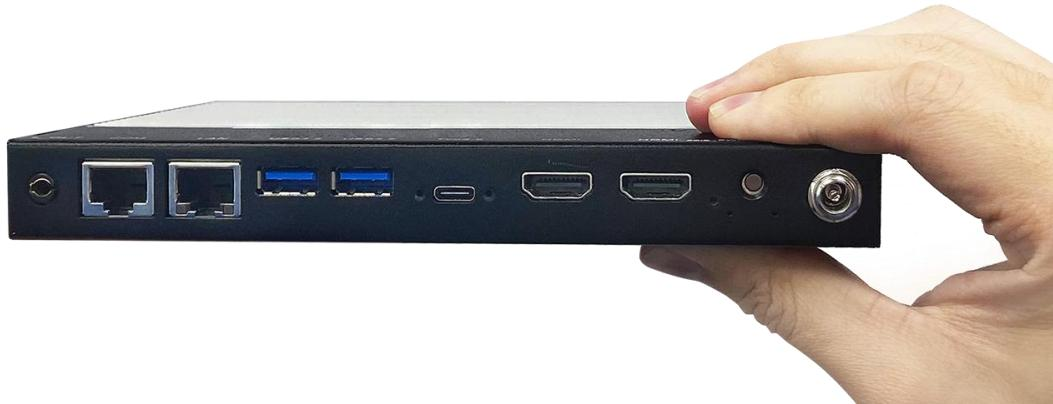
The SI-212-N also comes with IBASE's unique iSMART smart control energy-saving and Observer Connect remote monitoring & management technologies that feature automatic power on/off scheduling, automatic power recovery, low-temperature boot protection, hardware monitoring, and In-Band/Out-of-Band management. Standard features include 1x DDR5-4800 SO-DIMM, dual channel memory, max. 32GB, 1x M.2 E-key (2230) for WiFi or Bluetooth options, and TPM 2.0, vPro, and watchdog timer.
